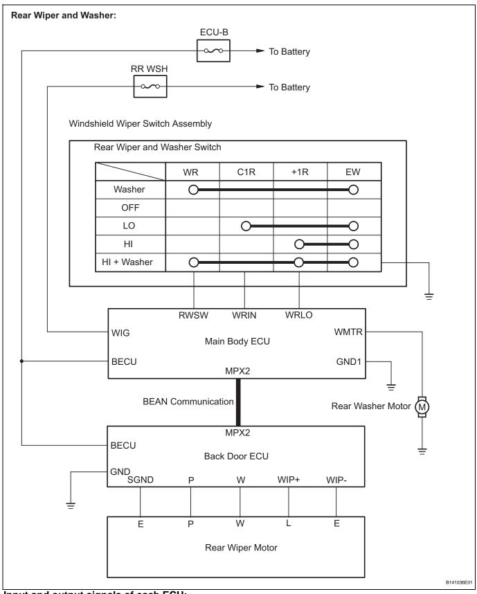
Input and output signals of each ECU:
